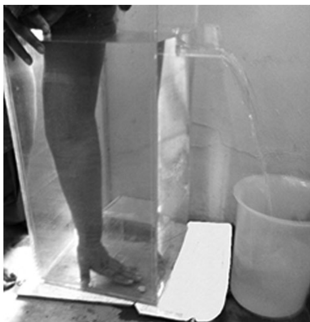
FIG. 1. Glass chamber along with the collecting glass cylinder with marking for measurement of displaced volume.
